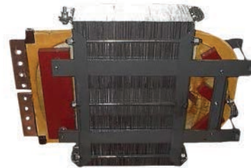
WELDING TRANSFORMER REPAIR 116 KVA, 480-5.8 to 11.6V
