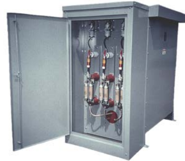
DRY NEMA 3R, 750 KVA, 5 KV, WITH Mc GRAW EDISON SW. BLADE AND FUSES, DIST. CLASS LIGHTNING ARRESTERS
